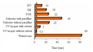
Fig. 2. Comparison of dryings time of coatings from selected lacquer products [6]
